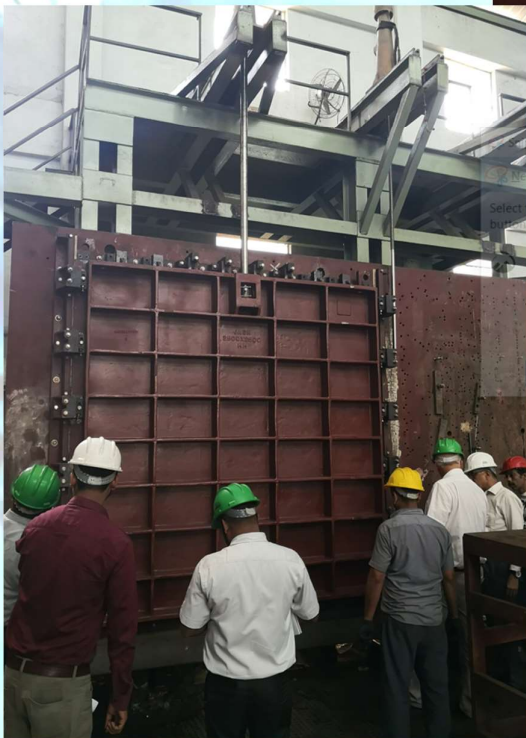
Jash cast iron penstock testing facility in Indore- India
